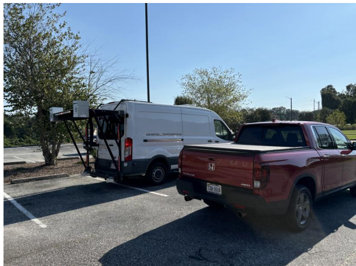
Laser profiler (left) and i-Probe SRMCV test vehicle (right)
